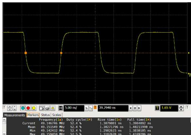
fosc=49.152MHz、 V_{DD} =3.3V、 C_L =15pF、Temp=25
