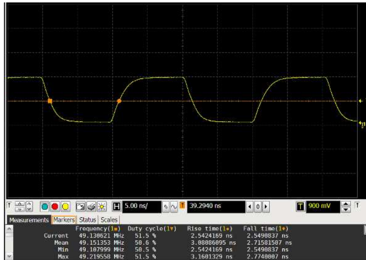
fosc=49.152MHz、 V_{DD} =1.8V、 C_L =15pF、Temp=25
