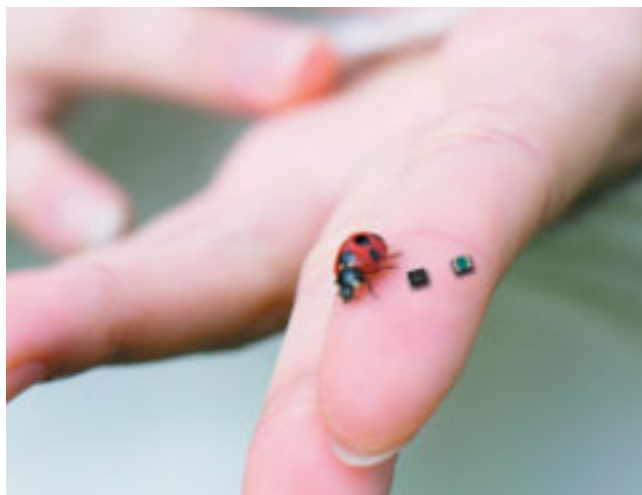
8 is a low noise amplifier designed mainly for one segment broadcasting. It features good gain flatness, and low gain characteristic in out-of-band in the UHF television band, achieving low current consumption, low noise figure and low harmonics. An ultra-small and ultra-thin package adopted.
