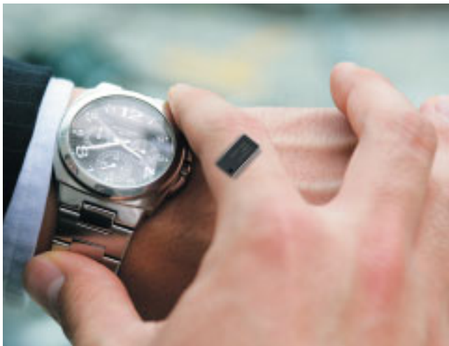
NJW1195 is a 4ch electronic volume with 4-input and 2-output selector. It features resistance ladder volume for low output noise voltage and low harmonics. Available as an electronic volume for 2ch differential transmission with 2-input and 1-output selector. Suitable for pure audio equipment such as player and amplifiers, AV amplifiers, and AV receivers.
