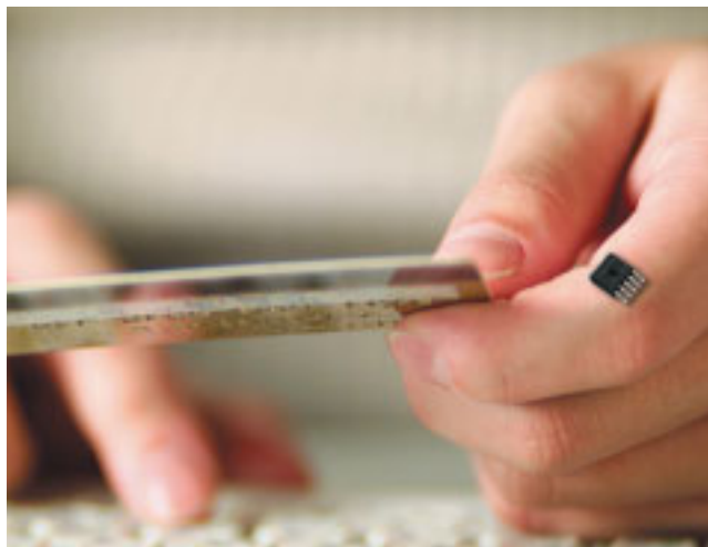
NJM2819 is a low noise and low saturation regulator with high-ripple rejection. It uses bipolar process and features output current of 2 A, most suitable for block requiring low input voltage and high output voltage.
