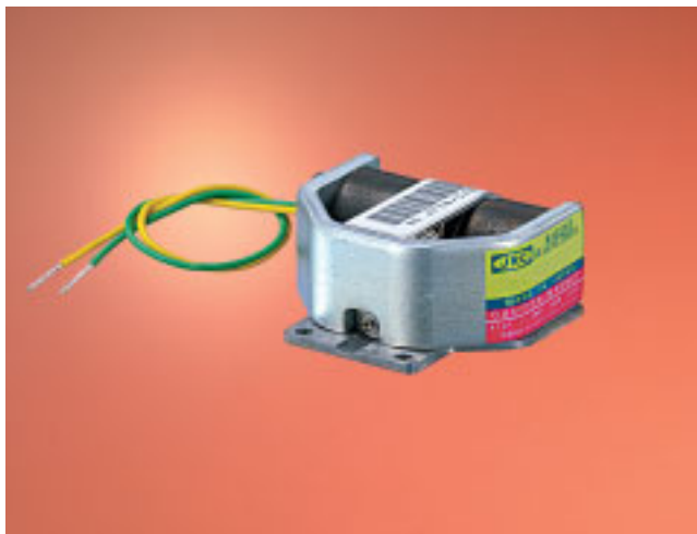
MAF1611B is an X-band magnetron for a marine radar. The peak output power is 4kW. Its spurious emission level is decreased and it outputs a clean X-band microwave.
