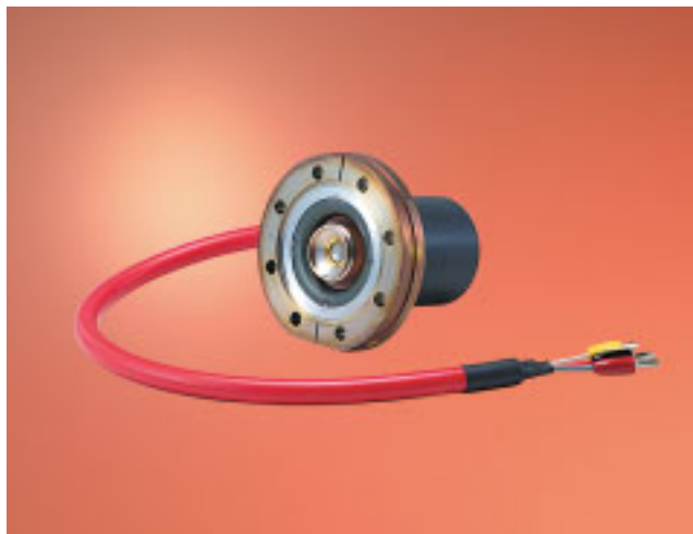
NJK2301 is an electron gun for a LINAC (Linear Accelerator) mainly used for a radiation therapy for cancer. An iridium-coated and Ba-impregnated cathode is installed into this electron gun and it achieves the operation with a high electron current density.
