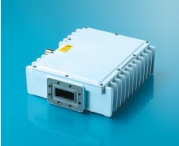
NJT5669 is a 5 to 6 GHz 5W output power transmitter, can be used to high speed and high capacity application for VSAT (Very Small Aperture Terminal) system of satellite communication, developed as generic product.
