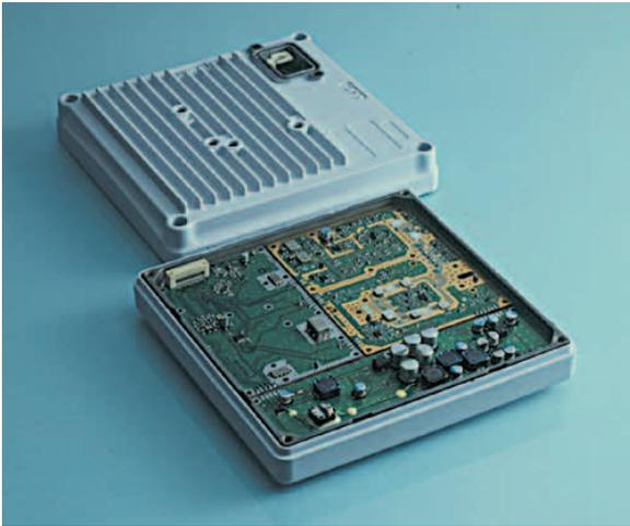
This is a compact subscriber station unit for 26 GHz FWA (Fixed Wireless Access) developed as an OEM product. Setup outside on a porch, etc., pointed at a base station enables a PC in house to access high-speed Internet services at 40 Mbps.
